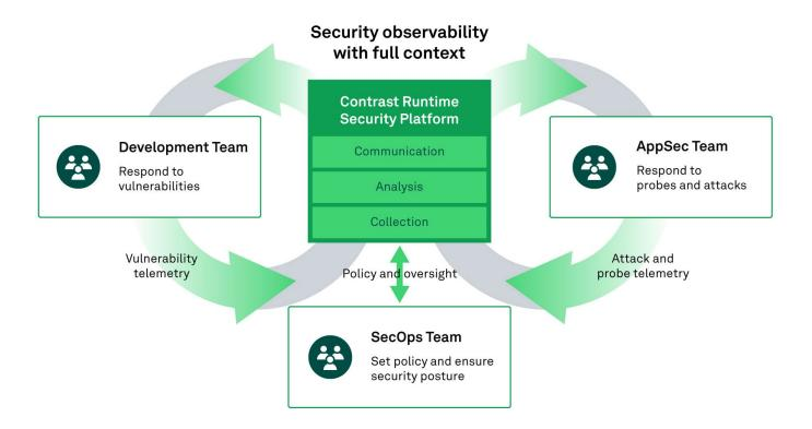
Figure 1: IAST in action: IAST identifies vulnerable code lines and risky data flows, providing full context. The development team addresses vulnerabilities, and the AppSec team monitors and responds to probes and attacks. Meanwhile, SecOps ensures overall security posture, creating a collaborative defense across development, application and operational layers.
